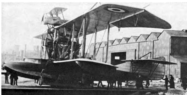
Bristol Scout hooked on the upper wing of a Felixstowe Porte Baby[sic] flying boat, 1916
